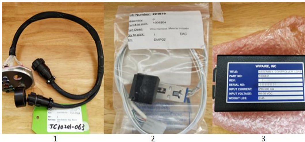
Figure 1: 1- landing gear control panel 21A11000-009, 2- landing gear master warning lights 1008204, 3- landing gear warning computer 1006831 )
